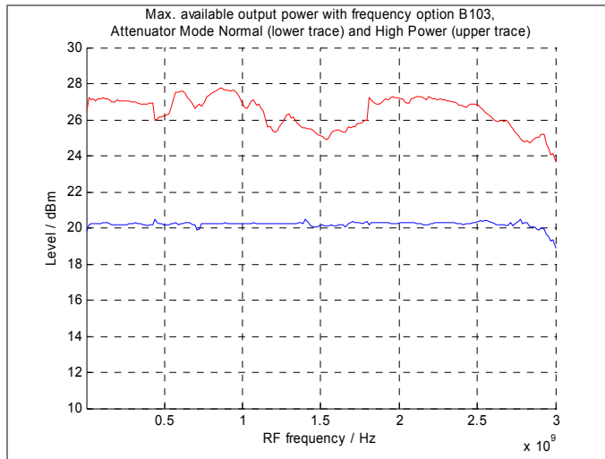
Measured maximum available output level versus frequency.
